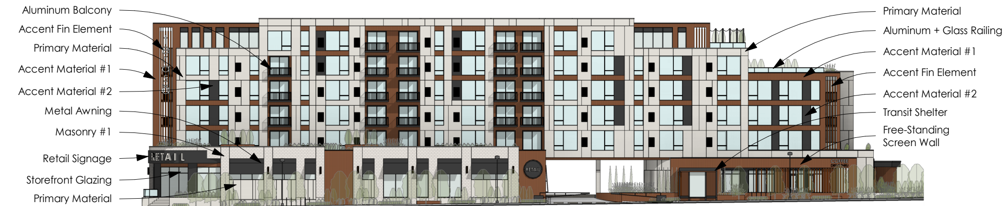
1 | West Elevation- Park Place Blvd. SCALE: 1" = 40'-0"
